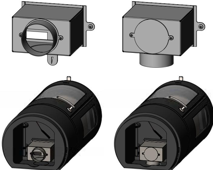
After fitting the required socket, the oven must be laid carefully on its rear, potentially on the packaging in which it arrived. The Fresh Air Box must be fitted to ensure that there is room for the air damper, which opens rearwards (see sketch).
