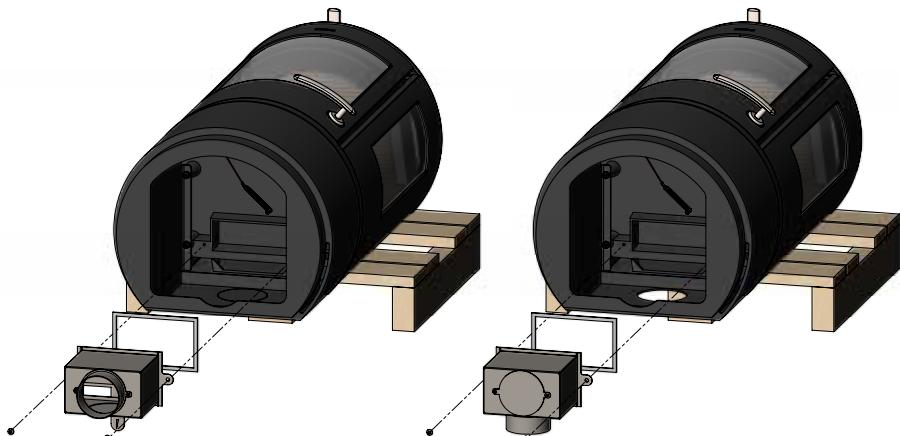
If the fresh air connection is to be fitted rearwards, the sheet steel panel on the rear of the socket must be knocked out with careful small blows by the small "bridges" that retain the panel.
